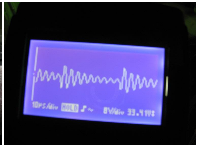
Scope reading of 33~37 peak-to-peak voltage
