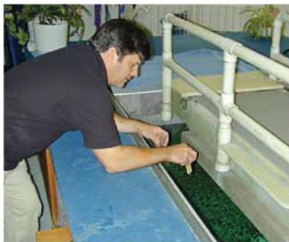
Owner Tom McCauley takes a measurement in one of the hydrotherapy pools using a dip slide.
