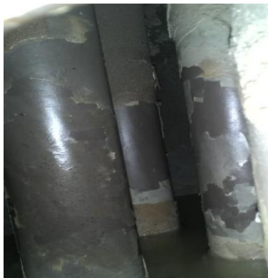
After 10 weeks - Bare tubes are beginning to show
